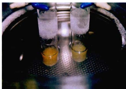
Figure 2. Lipase-catalyzed reactions at -40 °C in a cooling apparatus.
